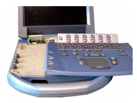
Figure 7.3 Control Panel Removal
