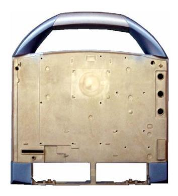
Figure A.4 Upper Enclosure, P05474 (top view)
