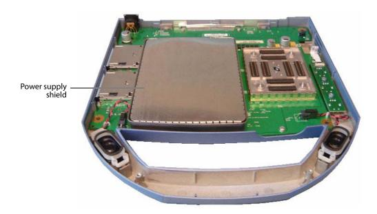
Figure 7.9 Power Supply Shield
